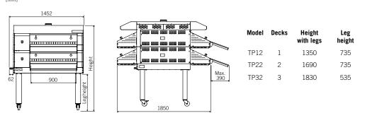
Infeed plate and outfeed plate are detachable, all models can be equipped with both infeed- and outfeed plates.
